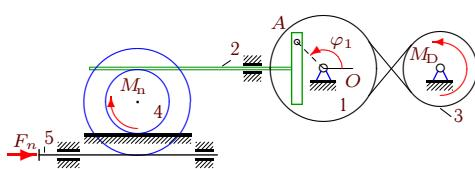
$$\begin{aligned}M_{Dz} &= M_0 - k\omega_{3z}, \\M_{nz} &= -\mu\omega_{4z}, \\F_{nx} &= -\nu v_{5x}, \\M_0 &= 13 \text{Нм}, k = 13 \text{Нмс}, \\&\nu = 8 \text{кНс/м}, \mu = 10 \text{Нмс}, \\I_1 &= 18 \text{кгм}^2, m_2 = 18 \text{кг}, \\m_3 &= 36 \text{кг}, m_4 = 28 \text{кг}, \\R_1 &= 36 \text{см}, r_1 = 25 \text{см}, \\R_3 &= 26 \text{см}, R_4 = 20 \text{см}, \\r_4 &= 12 \text{см}, i_4 = 17 \text{см}, \\&\varphi_{1,0} = 1.5, \omega_{1z,0} = 0.3 \frac{1}{c}.\end{aligned}$$
