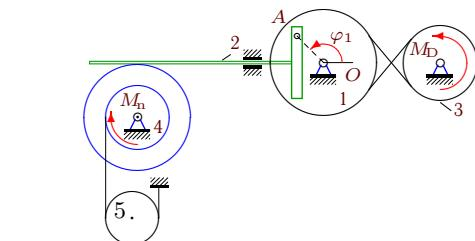
$$\begin{aligned}M_{Dz} &= M_0 - k\omega_{3z}, \\M_{nz} &= -\mu\omega_{4z}, \\M_0 &= 11 \text{Нм}, k = 13 \text{Нмс}, \\&\mu = 13 \text{Нмс}, I_1 = 12 \text{кгм}^2, \\m_2 &= 16 \text{кг}, m_3 = 34 \text{кг}, \\m_4 &= 26 \text{кг}, m_5 = 6 \text{кг}, \\R_1 &= 36 \text{см}, r_1 = 25 \text{см}, \\R_3 &= 26 \text{см}, R_4 = 20 \text{см}, \\r_4 &= 12 \text{см}, i_4 = 15 \text{см}, \\r_5 &= 12 \text{см}, \\&\varphi_{1,0} = 1.3, \omega_{1z,0} = 0.3 \frac{1}{c}.\end{aligned}$$
