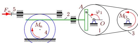
$$\begin{aligned}M_{Dz} &= M_0 - k\omega_{3z}, \\M_{nz} &= -\mu\omega_{4z}, \\F_{nx} &= -\nu v_{5x}, \\M_0 &= 10 \text{Нм}, k = 15 \text{Нмс}, \\I_1 &= 9 \text{кгм}^2, m_2 = 16 \text{кг}, \\m_3 &= 34 \text{кг}, m_4 = 26 \text{кг}, \\R_1 &= 38 \text{см}, r_1 = 27 \text{см}, \\R_3 &= 28 \text{см}, R_4 = 20 \text{см}, \\r_4 &= 12 \text{см}, i_4 = 15 \text{см}, \\&\varphi_{1,0} = 1.3, \omega_{1z,0} = 0.5 \frac{1}{c}.\end{aligned}$$
