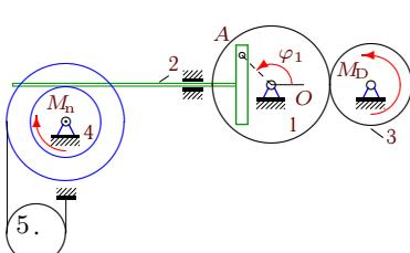
$$\begin{aligned}M_{Dz} &= M_0 - k\omega_{3z}, \\M_{nz} &= -\mu\omega_{4z}, \\M_0 &= 10 \text{Нм}, k = 13 \text{Нмс}, \\&\mu = 11 \text{Нмс}, I_1 = 7 \text{кгм}^2, \\m_2 &= 17 \text{кг}, m_3 = 35 \text{кг}, \\m_4 &= 27 \text{кг}, m_5 = 4 \text{кг}, \\R_1 &= 36 \text{см}, r_1 = 25 \text{см}, \\R_3 &= 26 \text{см}, R_4 = 20 \text{см}, \\r_4 &= 12 \text{см}, i_4 = 16 \text{см}, \\r_5 &= 10 \text{см}, \\&\varphi_{1,0} = 1.4, \omega_{1z,0} = 0.3 \frac{1}{с}.\end{aligned}$$
