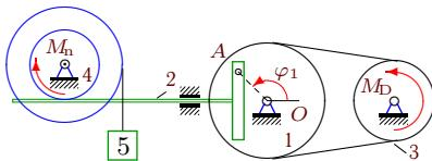
$$\begin{aligned}M_{Dz} &= M_0 - k\omega_{3z}, \\M_{nz} &= -\mu\omega_{4z}, \\M_0 &= 10 \text{Нм}, k = 15 \text{Нмс}, \\&\mu = 12 \text{Нмс}, I_1 = 9 \text{кгм}^2, \\m_2 &= 16 \text{кг}, m_3 = 34 \text{кг}, \\m_4 &= 26 \text{кг}, m_5 = 4 \text{кг}, \\R_1 &= 38 \text{см}, r_1 = 27 \text{см}, \\R_3 &= 28 \text{см}, R_4 = 20 \text{см}, \\r_4 &= 12 \text{см}, i_4 = 15 \text{см}, \\&\varphi_{1,0} = 1.3, \omega_{1z,0} = 0.5 \frac{1}{с}.\end{aligned}$$
