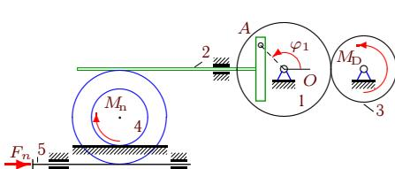
$$\begin{aligned}M_{Dz} &= M_0 - k\omega_{3z}, \\M_{nz} &= -\mu\omega_{4z}, \\F_{nx} &= -\nu v_{5x}, \\M_0 &= 9 \text{Нм}, k = 12 \text{Нмс}, \\&\nu = 8 \text{кНс/м}, \mu = 12 \text{Нмс}, \\I_1 &= 6 \text{кгм}^2, m_2 = 16 \text{кг}, \\m_3 &= 34 \text{кг}, m_4 = 26 \text{кг}, \\R_1 &= 35 \text{см}, r_1 = 24 \text{см}, \\R_3 &= 25 \text{см}, R_4 = 20 \text{см}, \\r_4 &= 12 \text{см}, i_4 = 15 \text{см}, \\&\varphi_{1,0} = 1.3, \omega_{1z,0} = 0.2 \frac{1}{с}.\end{aligned}$$
