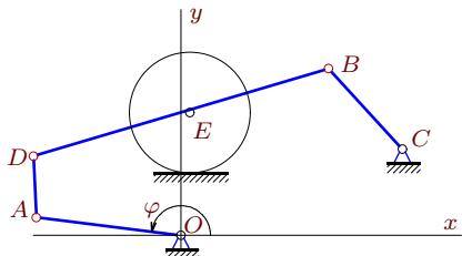
$$\begin{aligned}\omega_{OA_z} &= -5 \text{ рад/c, } BC = 10, \\ DE &= BE = 13, OA = 12, \\ AD &= 5, x_C = 18, y_C = 7, \\ y_E &= 10, \varphi_0 = \pi.\end{aligned}$$
