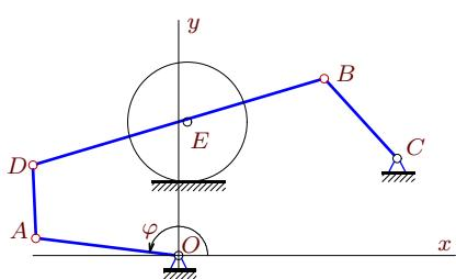
$$\begin{aligned}\omega_{OA_z} &= -3 \text{ рад/с}, \quad BC = 10, \\ DE &= BE = 13, \quad OA = 12, \\ AD &= 6, \quad x_C = 18, \quad y_C = 8, \\ y_E &= 11, \quad \varphi_0 = \pi.\end{aligned}$$
