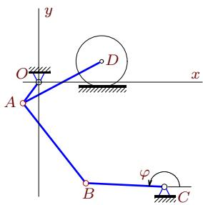
$v_{Dx} = -48 \text{ см/с}, OA = 5, AB = 20, BC = 15, AD = 17, x_C = 24, y_C = -20, y_D = 4, \varphi_0 = \pi.$
