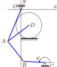
$$\begin{aligned}\omega_{BC_z} &= 14 \text{ рад/с}, OA = 13, \\ AB &= 10, BC = 8, AD = 10, \\ x_C &= 9, y_C = -20, y_D = -6, \\ \varphi_0 &= \pi.\end{aligned}$$
