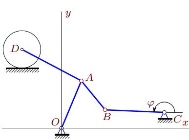
$v_{Dx} = -440 \text{ см/с}, OA = 13, AB = 10, BC = 15, AD = 17, x_C = 26, y_C = 4, y_D = 20, \varphi_0 = \pi.$
