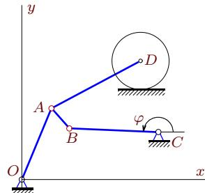
$$\begin{aligned} \omega_{BCz} &= -14 \text{ rad/c}, OA = 13, \\ AB &= 5, BC = 15, AD = 17, \\ x_C &= 23, y_C = 8, y_D = 20, \\ \varphi_0 &= \pi. \end{aligned}$$
