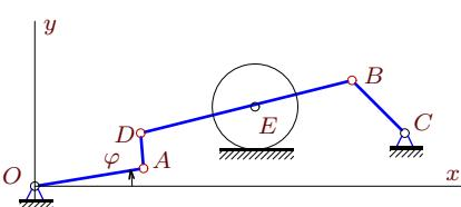
$$\begin{aligned}\omega_{OA_z} &= 2 \text{ rad/c}, \quad BC = 10, \\ DE &= BE = 13, \quad OA = 12, \\ AD &= 4, \quad x_C = 42, \quad y_C = 6, \\ y_E &= 9, \quad \varphi_0 = 0.\end{aligned}$$
