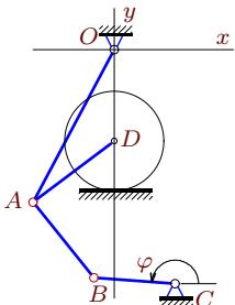
$$\begin{aligned}\omega_{OA_z} &= 32 \text{ рад/с}, OA = 17, \\ AB &= 10, BC = 8, AD = 10, \\ x_C &= 6, y_C = -23, y_D = -9, \\ \varphi_0 &= \pi.\end{aligned}$$
