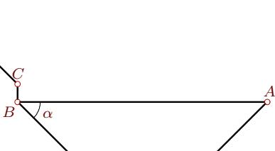
$\omega_{OA_z} = -7\frac{1}{c}$ ,  $\omega_{CF_z} = -14\frac{1}{c}$ ,  $AB = 14$ ,  $BC = 1$ ,  $DE = 4$ ,  $OA = CF = BD = 4\sqrt{2}$ ,  $\alpha = 45^\circ$ .
