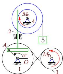
$$\begin{aligned}M_{Dz} &= M_0 - k\omega_{3z}, \\M_{nz} &= -\mu\omega_{4z}, \\M_0 &= 13 \text{Нм}, k = 14 \text{Нмс}, \\&\mu = 10 \text{Нмс}, I_1 = 18 \text{кгм}^2, \\m_2 &= 18 \text{кг}, m_3 = 36 \text{кг}, \\m_4 &= 28 \text{кг}, m_5 = 7 \text{кг}, \\R_1 &= 37 \text{см}, r_1 = 26 \text{см}, \\R_3 &= 27 \text{см}, R_4 = 20 \text{см}, \\r_4 &= 12 \text{см}, i_4 = 17 \text{см}, \\&\varphi_{1,0} = 1.5, \omega_{1z,0} = 0.4 \frac{1}{c}.\end{aligned}$$
