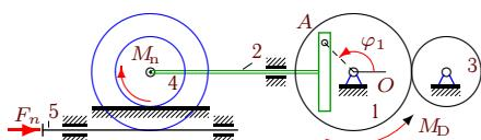
$$\begin{aligned}M_{Dz} &= M_0 - k\omega_{1z}, \\M_{nz} &= -\mu\omega_{4z}, \\F_{nx} &= -\nu v_{5x}, \\M_0 &= 10 \text{Нм}, k = 11 \text{Нмс}, \\&\nu = 8 \text{кНс/м}, \mu = 14 \text{Нмс}, \\I_1 &= 7 \text{кгм}^2, m_2 = 14 \text{кг}, \\m_3 &= 32 \text{кг}, m_4 = 24 \text{кг}, \\R_1 &= 34 \text{см}, r_1 = 23 \text{см}, \\R_3 &= 24 \text{см}, R_4 = 20 \text{см}, \\r_4 &= 12 \text{см}, i_4 = 13 \text{см}, \\&\varphi_{1,0} = 1.1, \omega_{1z,0} = 0.1 \frac{1}{c}.\end{aligned}$$
