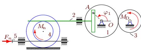
$$\begin{aligned}M_{Dz} &= M_0 - k\omega_{3z}, \\M_{nz} &= -\mu\omega_{4z}, \\F_{nx} &= -\nu v_{5x}, \\M_0 &= 9 \text{Нм}, k = 15 \text{Нмс}, \\I_1 &= 6 \text{кгм}^2, m_2 = 16 \text{кг}, \\m_3 &= 34 \text{кг}, m_4 = 26 \text{кг}, \\R_1 &= 38 \text{см}, r_1 = 27 \text{см}, \\R_3 &= 28 \text{см}, R_4 = 20 \text{см}, \\r_4 &= 12 \text{см}, i_4 = 15 \text{см}, \\&\varphi_{1,0} = 1.3, \omega_{1z,0} = 0.5 \frac{1}{c}.\end{aligned}$$
