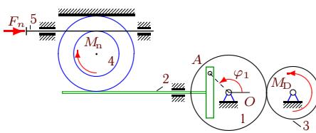
$$\begin{aligned}M_{Dz} &= M_0 - k\omega_{3z}, \\M_{nz} &= -\mu\omega_{4z}, \\F_{nx} &= -\nu v_{5x}, \\M_0 &= 9 \text{Нм}, k = 11 \text{Нмс}, \\&\nu = 8 \text{кНс/м}, \mu = 13 \text{Нмс}, \\I_1 &= 6 \text{кгм}^2, m_2 = 16 \text{кг}, \\m_3 &= 34 \text{кг}, m_4 = 26 \text{кг}, \\R_1 &= 34 \text{см}, r_1 = 23 \text{см}, \\R_3 &= 24 \text{см}, R_4 = 20 \text{см}, \\r_4 &= 12 \text{см}, i_4 = 15 \text{см}, \\&\varphi_{1,0} = 1.3, \omega_{1z,0} = 0.1 \frac{1}{c}.\end{aligned}$$
