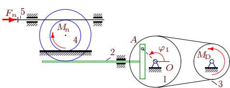
$$\begin{aligned}M_{Dz} &= M_0 - k\omega_{3z}, \\M_{nz} &= -\mu\omega_{4z}, \\F_{nx} &= -\nu v_{5x}, \\M_0 &= 12 \text{Нм}, k = 15 \text{Нмс}, \\&\nu = 35 \text{кНс/м}, \mu = 10 \text{Нмс}, \\I_1 &= 13 \text{кгм}^2, m_2 = 18 \text{кг}, \\m_3 &= 36 \text{кг}, m_4 = 28 \text{кг}, \\R_1 &= 38 \text{см}, r_1 = 27 \text{см}, \\R_3 &= 28 \text{см}, R_4 = 20 \text{см}, \\r_4 &= 12 \text{см}, i_4 = 17 \text{см}, \\&\varphi_{1,0} = 1.5, \omega_{1z,0} = 0.5 \frac{1}{c}.\end{aligned}$$
