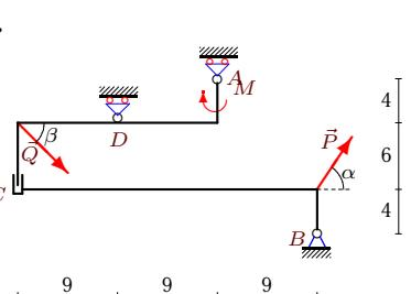
$$P = 40 \text{ kH}, Q = 50 \text{ kH}, \alpha = 60^\circ, \\ \beta = 45^\circ, \rho = 4 \text{ kH/m}, M = 100 \text{ kNm}.$$
