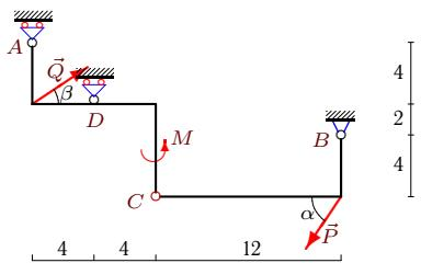
$P = 20 \text{ kH}$ ,  $Q = 30 \text{ kH}$ ,  $\alpha = 60^\circ$ ,
