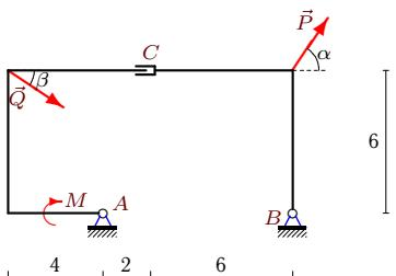
$P = 20 \text{ kH}$ ,  $Q = 30 \text{ kH}$ ,  $\alpha = 60^\circ$ ,
