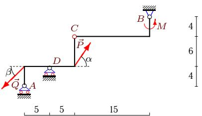
$P = 40 \text{ кН}$ ,  $Q = 50 \text{ кН}$ ,  $\alpha = 60^\circ$ ,
