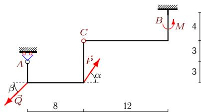
$P = 40 \text{ kH}$ ,  $Q = 50 \text{ kH}$ ,  $\alpha = 60^\circ$ ,
