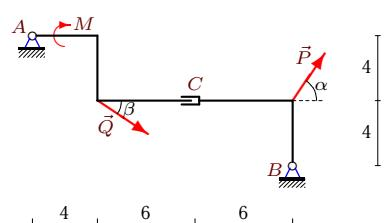
$$P = 20 \text{ кН}, Q = 30 \text{ кН}, \alpha = 60^\circ, \beta = 30^\circ, \rho = 2 \text{ кН/м}, M = 80 \text{ кНм}.$$
