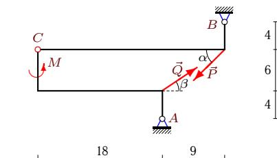
$P = 50 \text{ kH}$ ,  $Q = 60 \text{ kH}$ ,  $\alpha = 45^\circ$ ,
