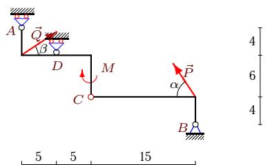
$$P = 20 \text{ kH}, Q = 30 \text{ kH}, \alpha = 60^\circ, \\ \beta = 30^\circ, \rho = 3 \text{ kH/m}, M = 130 \text{ kHm}.$$
