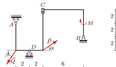
$P = 10 \text{ kH}$ ,  $Q = 20 \text{ kH}$ ,  $\alpha = 30^\circ$ ,
