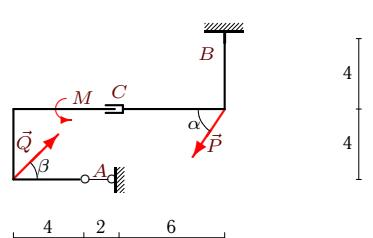
$$P = 40 \text{ kH}, Q = 50 \text{ kH}, \alpha = 60^\circ, \\ \beta = 45^\circ, \rho = 6 \text{ kH/m}, M = 80 \text{ kNm}.$$
