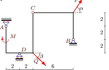
$$P = 40 \text{ кН}, Q = 50 \text{ кН}, \alpha = 60^\circ, \beta = 45^\circ, \rho = 3 \text{ кН/м}, M = 40 \text{ кНм}.$$
