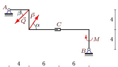
$P = 40 \text{ kH}$ ,  $Q = 50 \text{ kH}$ ,  $\alpha = 60^\circ$ ,
