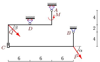
$P = 40 \text{ кН}$ ,  $Q = 50 \text{ кН}$ ,  $\alpha = 60^\circ$ ,
