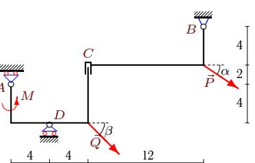
$$P = 30 \text{ kH}, Q = 40 \text{ kH}, \alpha = 30^\circ, \\ \beta = 45^\circ, \rho = 4 \text{ kH/m}, M = 40 \text{ kHm}.$$
