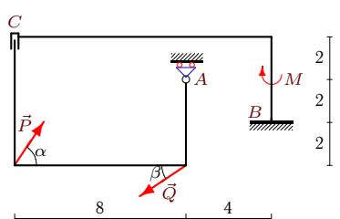
$$P = 20 \text{ kH}, Q = 30 \text{ kH}, \alpha = 60^\circ, \\ \beta = 30^\circ, \rho = 6 \text{ kH/m}, M = 10 \text{ kHM}.$$
