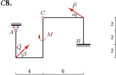
$P = 30 \text{ kH}$ ,  $Q = 40 \text{ kH}$ ,  $\alpha = 30^\circ$ ,
