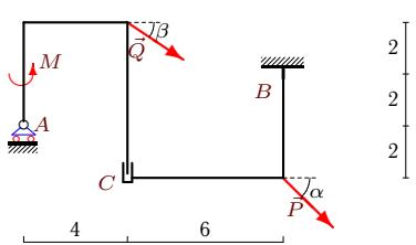
$$P = 50 \text{ кН}, Q = 60 \text{ кН}, \alpha = 45^\circ, \beta = 30^\circ, \rho = 6 \text{ кН/м}, M = 130 \text{ кНм}.$$
