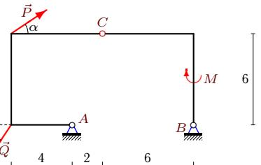
$$P = 10 \text{ kH}, Q = 20 \text{ kH}, \alpha = 30^\circ, \\ \beta = 60^\circ, \rho = 1 \text{ kH/m}, M = 60 \text{ kNm}.$$
