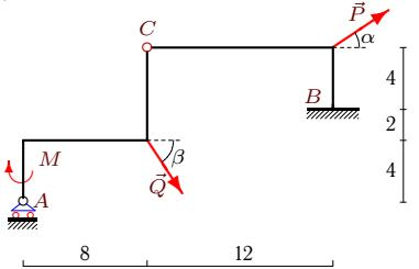
$$P = 10 \text{ кН}, Q = 20 \text{ кН}, \alpha = 30^\circ, \beta = 60^\circ, \rho = 5 \text{ кН/м}, M = 50 \text{ кНм}.$$
