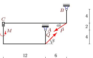
$$P = 30 \text{ kH}, Q = 40 \text{ kH}, \alpha = 30^\circ, \\ \beta = 45^\circ, \rho = 2 \text{ kH/m}, M = 30 \text{ kHm}.$$
