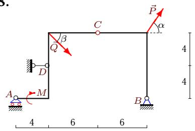
$P = 40 \text{ кН}$ ,  $Q = 50 \text{ кН}$ ,  $\alpha = 60^\circ$ ,
