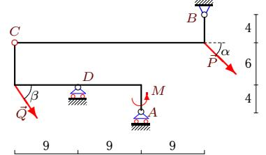
$$P = 60 \text{ кН}, Q = 70 \text{ кН}, \alpha = 45^\circ, \beta = 60^\circ, \rho = 3 \text{ кН/м}, M = 30 \text{ кНм}.$$
