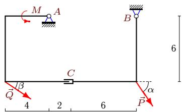
$$P = 20 \text{ кН}, Q = 30 \text{ кН}, \alpha = 60^\circ, \beta = 30^\circ, \rho = 2 \text{ кН/м}, M = 90 \text{ кНм}.$$
