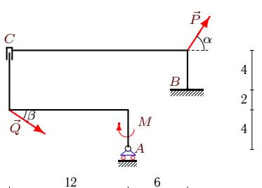
$$P = 20 \text{ kH}, Q = 30 \text{ kH}, \alpha = 60^\circ, \\ \beta = 30^\circ, \rho = 6 \text{ kH/m}, M = 30 \text{ kHm}.$$
